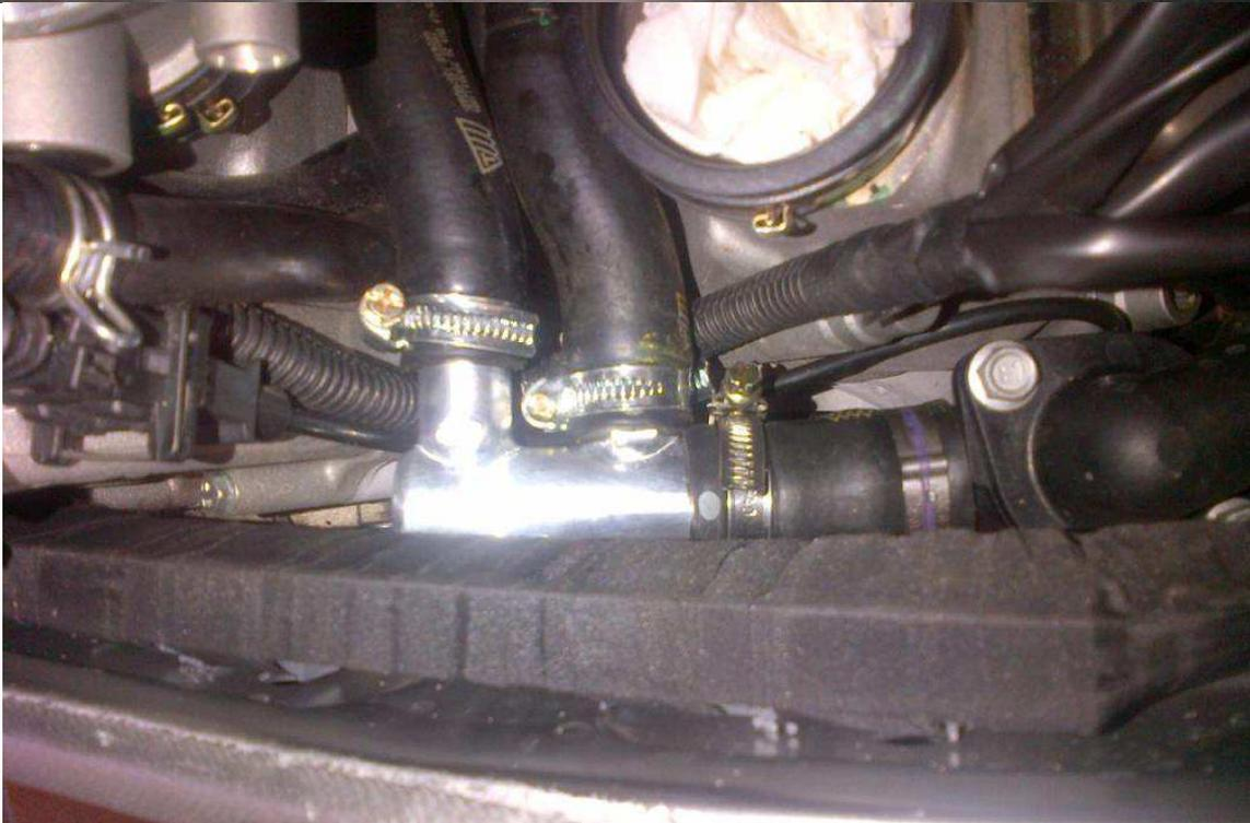
19. To reassemble the "Click" clamps of throttle body, instead of expensive Aprilia pliers, you can modify a pair of cheaper pliers (45° bent), as indicated in the pictures (I have grinded the ends as wedge shape; on the left end I have practiced an incision, that correspond to the clamp rib):
