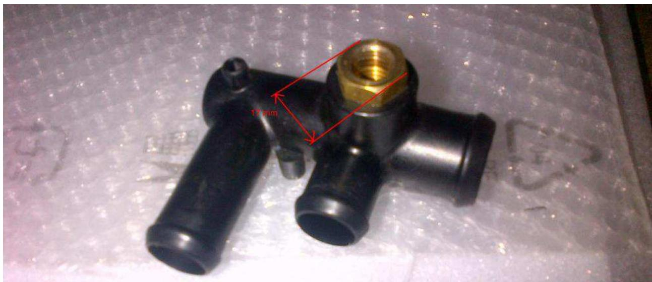
16. Install the sensor on the cnc manifold:
