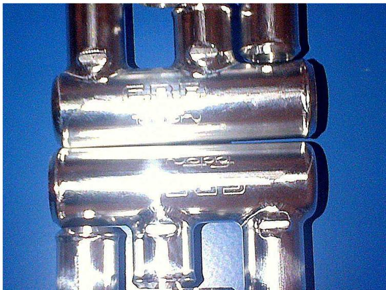
After you have remove seat, right fairing, left and right underseat fairings, fuel tank, here the tools you'll need to replace the original plastic part with cnc manifold:
