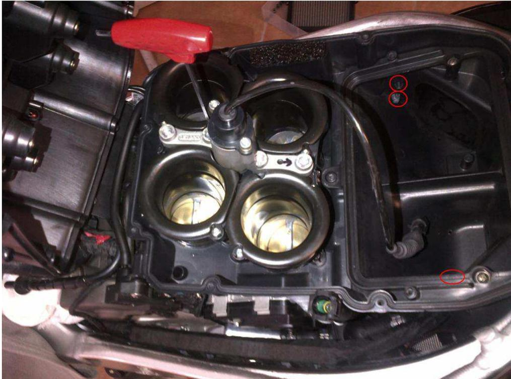
5. On the left side of motorcycle, under the airbox, disconnect a clip that fixes wiring to a bracket:
