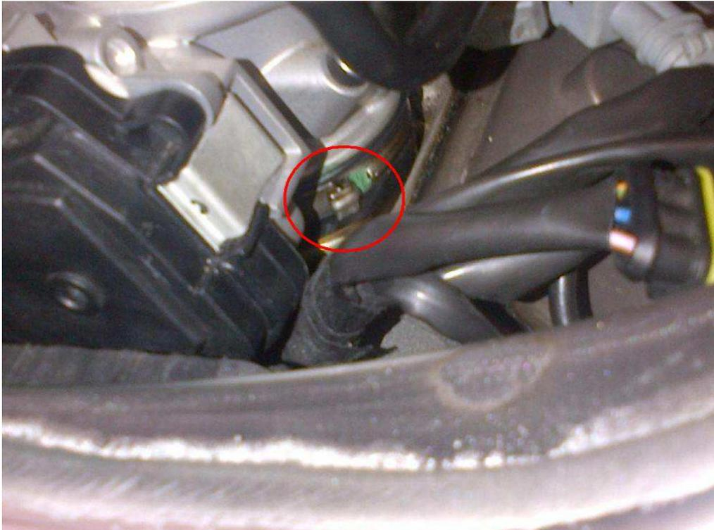
10. Disconnect the injectors connectors (enlarge the metal wire clip with tool "C" on the red circled zone):
