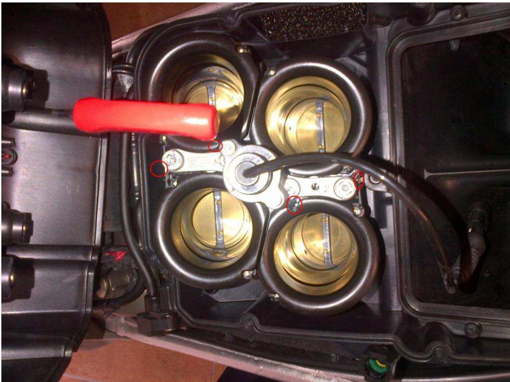
Remove the variable geometry connector from the airbox cover.
