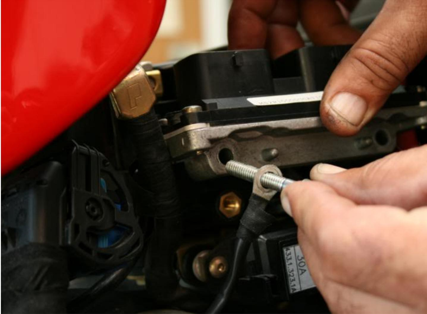
Now to reinstall it. Don't forget to put the ground wire on this bolt.
