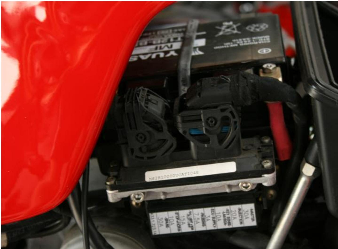
The harnesses that connect to the ECU are secured in place by these clips that you must push down.
