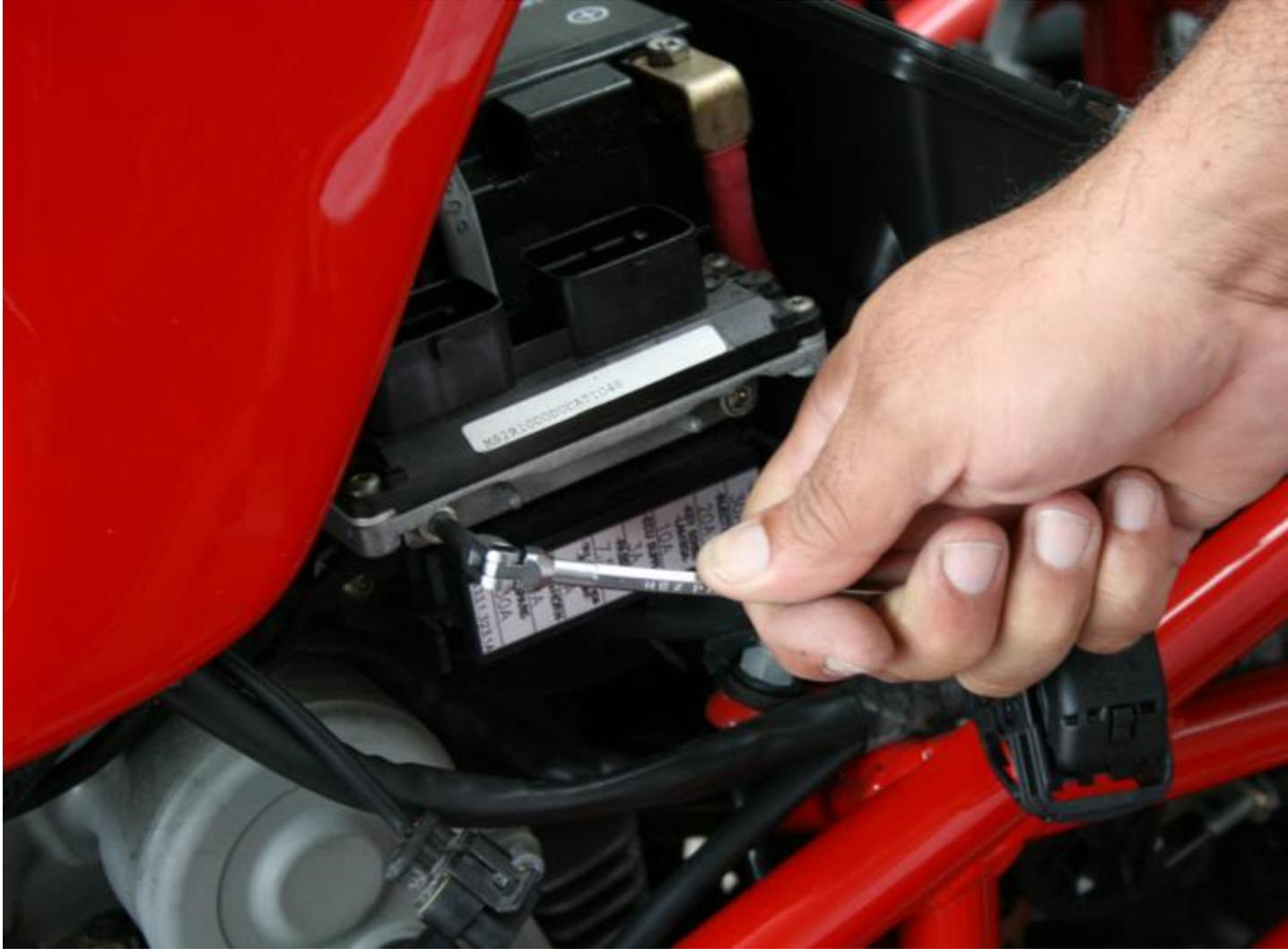
Remove the screws securing it in place.
