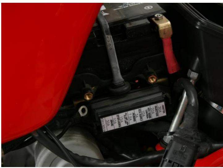
And remove the ECU. Note the ground wire.
